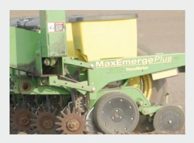
If your planter's a 3-point mounted planter you're going to want to adjust the lift arms to get the quick hitch leveled before hooking up the planter. If you have draft control on your tractor, you're going to want to turn that down or off before planting to make sure it's not trying to adjust that height and the levelness of the planter when you're going through the field.
