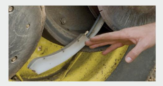
When a seed comes down the seed tube and into the furrow, you want it to get to the bottom of the furrow, not be hung up with an air pocket underneath it. A Keeton® Seed Firmer on each row will press the seed down to the bottom of the trench to get into moisture, helping you achieve consistent germination.
