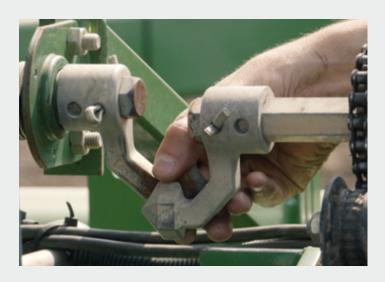
Vibration caused by mechanical components like chains and sprockets can take a properly performing meter and cause it to create skips, doubles, and spacing errors. Be sure to check the following components for wear:
