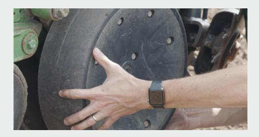
Uniform emergence means that every single seed needs to be in the same moisture environment. One part of the planter that can affect this negatively is poor shimming of the gauge wheel.
