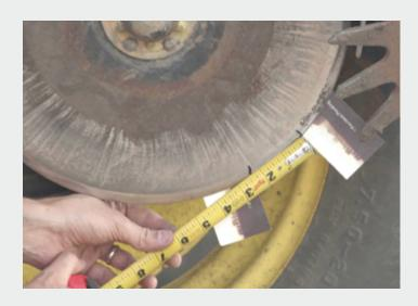
Disk openers create the furrow that seeds are placed in. To make sure that this process happens properly, you have to keep up with maintenance. Disk openers that are not maintained properly will cause erratic emergence and lost yield.
