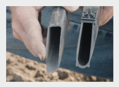
Get a tape measure and measure your guards. You want your guards to be at least ¾ of an inch wide at the start of a new season. If it's less than that it's time to replace that seed tube guard with a new one, which is 15/16 inches wide. You should always replace the seed tube guards when you're putting a new set of opener disks on the planter.
